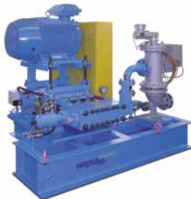
Pump unit DP 207 for the descaling of copper.
