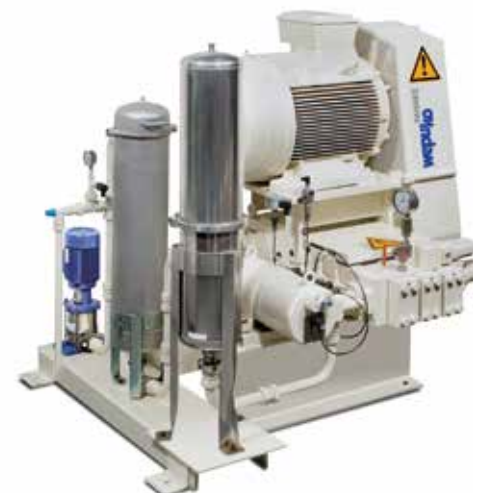
Compact version of the pump unit DP 405 for the cooling of tools including booster pump and filters (suction side) and resonator for pressure pulsation dampening (pressure side).
