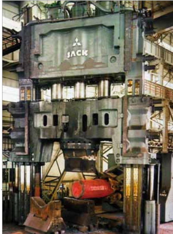
100 MN press for Japan Casting & Forging (1972): clamped columns screwed to the cross head
