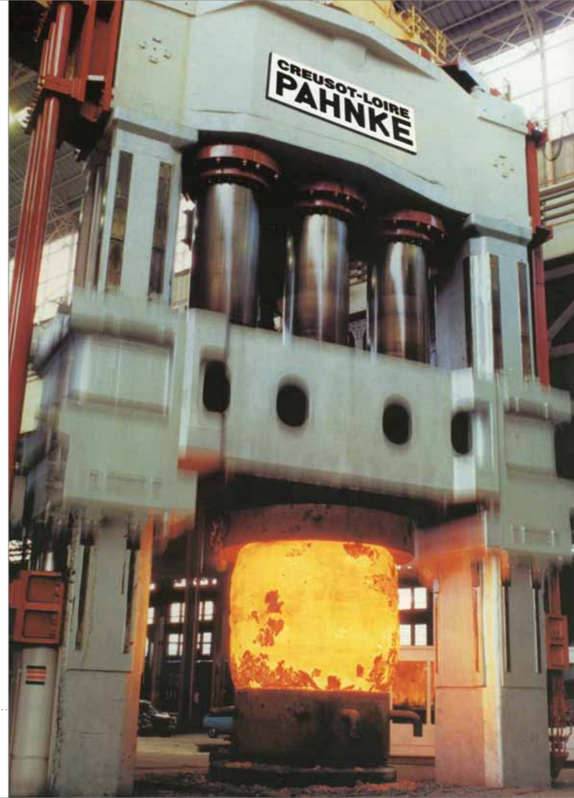
PAHNKE Engineering for Creusot-Loire (1976): 110 MN press with several tie rods per column (= pre-tensioned frame)
