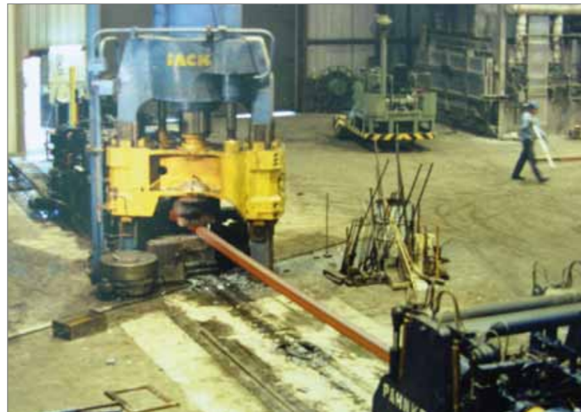
One of Michael Pahnke's projects at PSI (1979): PMSD drive, two manipulators and new control for a 7 MN press at Press Forge Co.
