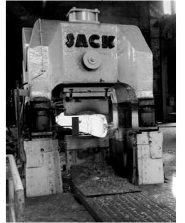
6.3 MN "Mannheim" under floor press (1961)
