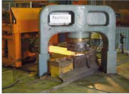
5 MN pull down open die forging press for MEFOS (first PAHNKE press and first Pahnke Modified Sinusoidal Direct Drive)
