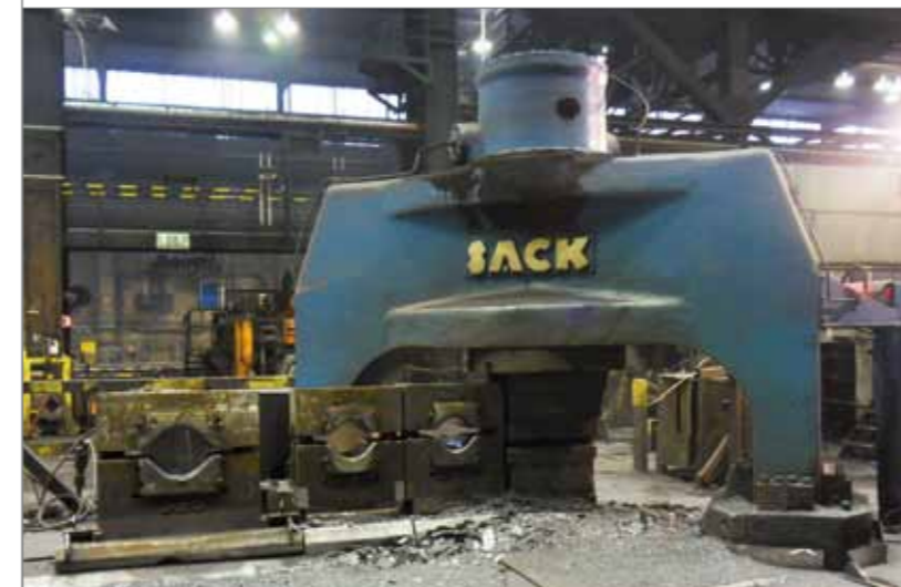
SACK open die press with two-column construction
