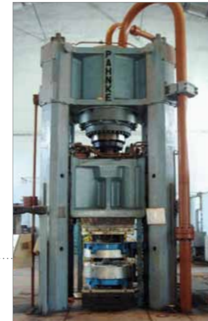
20 MN isothermal press with power levels of 15 and 6 MN with in-built ISO tools (1986)
