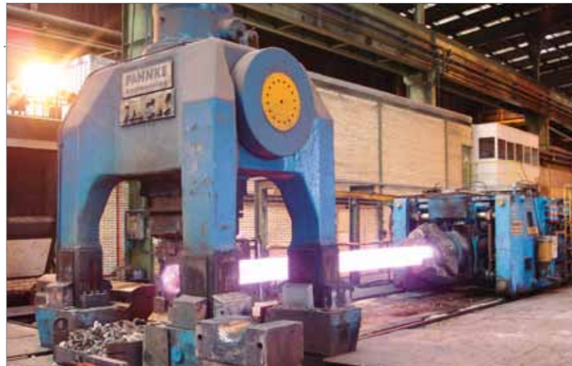
20 MN press for Latrobe Steel (1966 to 1995). Has been in use in Aceralava (Tubacex) in Spain since 1997 – modernised and converted from valve control to PMSD system with 10 RX 250 pumps
