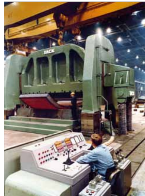
The 120 MN bending press from SACK: The design on the left and in use on the right
