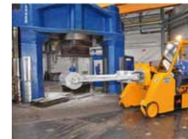
Weber open die press (same construction as the press for Fuchs) with PMSD drive (2009)
